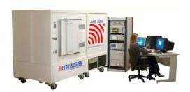
ETS-Lindgren's Model AMS-8050 Antenna Measurement System supports testing a wide range of portable wireless devices and mobile handsets in free-space or using a head and hands phantoms. The AMS-8050 is a compact, fully anechoic RF enclosure for over-the-air (OTA) testing. It is used for wireless device measurements including precertification testing, design verification, performance verification, and production sample testing.
